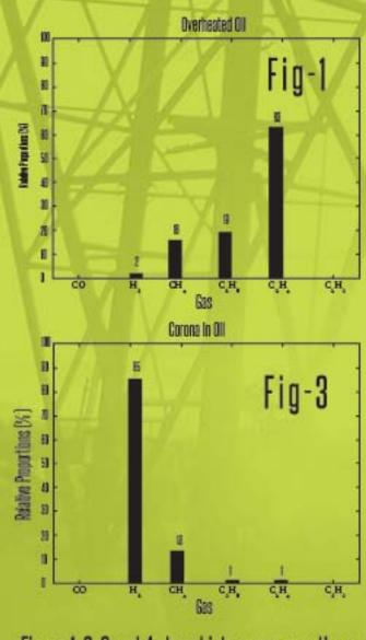
Figure-1, 2, 3 and 4 show histograms over the main decomposition products for each of the four fault types.
